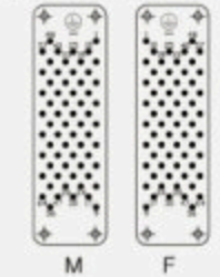
面板安装开孔图 Panel cut out for inserts for use without Hood/housings
