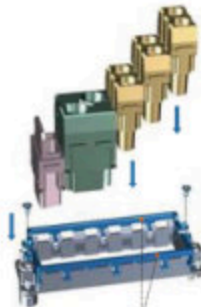
装配前松开滑动边框 Loosen sliding border before assembly
