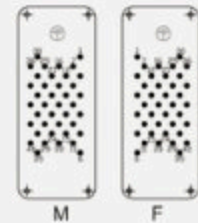
面板安装开孔图 Panel cut out for inserts for use without Hood/housings
